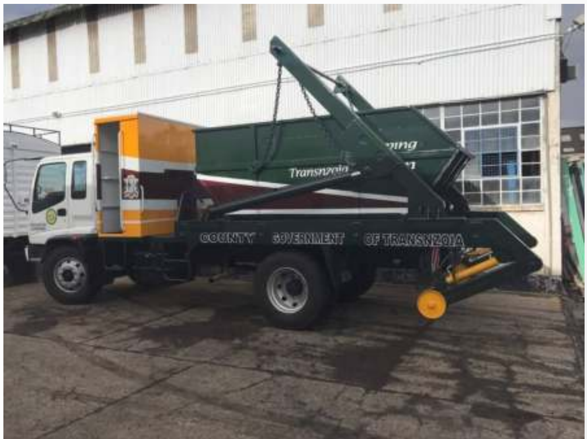
Figure 18: Procured Skip loader
